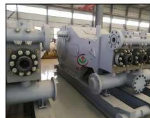
Cementing Pump Skid Overview
