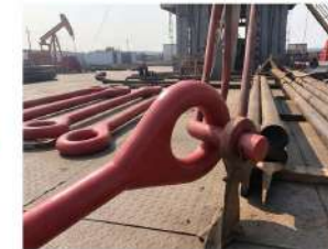
Elevator Body Detail
