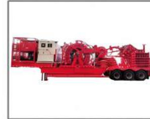
Coiled Tubing Unit
