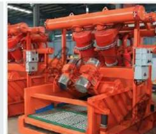
MUD CLEANER COMPLETE UNIT (BWwell)
